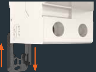
Bi Stable Clip Every device is provided with a dual position DIN rail clip, so it becomes much easier to change a device from a device bank connected to a bus-bar, without disturbing the existing wiring
